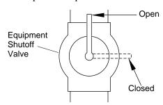
Figure 13 - Equipment Shutoff Valve
